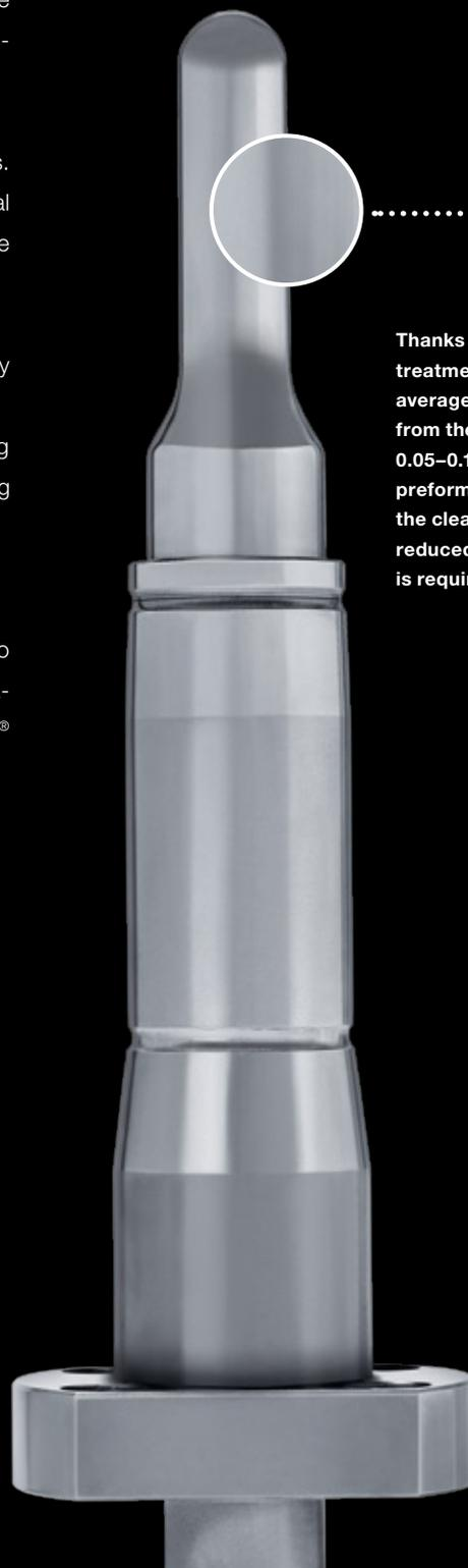
Thanks to the newly developed surface treatment OH-Xtra®, the arithmetic average of roughness (Ra) is reduced from the traditional 0.2–0.3 µm to a mere 0.05–0.1 µm. This means that the preforms are free of micro-scratches, the cleaning effort in the mould is reduced and a lower ejection force is required.
